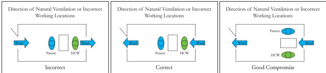
Directional air flow should be maintained from a “clean” area, across the HCW, across the patient, and to the outside. The area where air is entering should be located away from the exhaust area to avoid re-entry of contaminated air.
